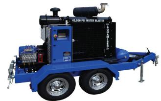
Optional pump conversion package available for 6 gpm at 25,000 psi.
